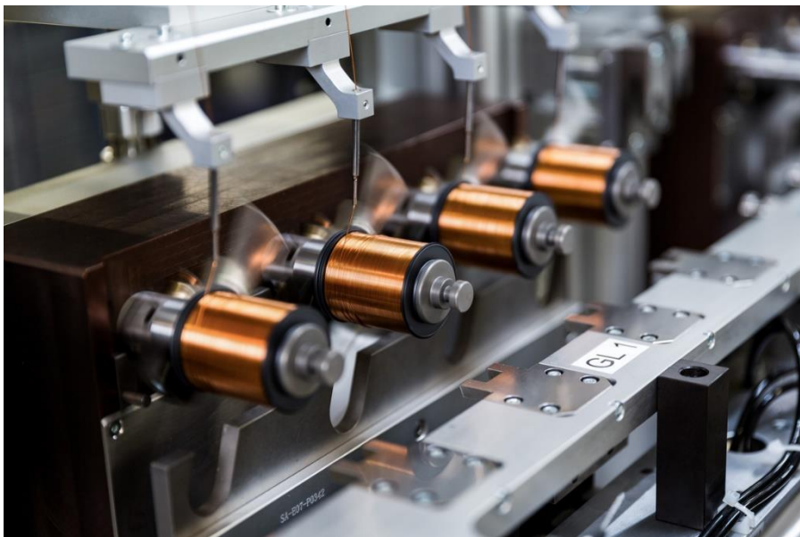
The KUK winding module developed by KUK is the heart of the production line. It is also used as a modular system for other projects.
